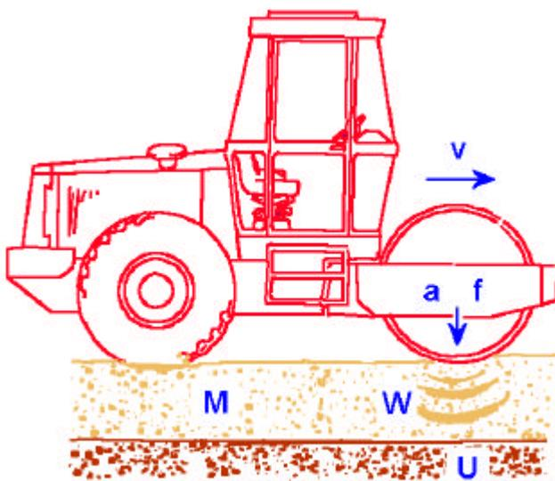
**Figure 1.** Constant roller parameters and varying ground conditions.
