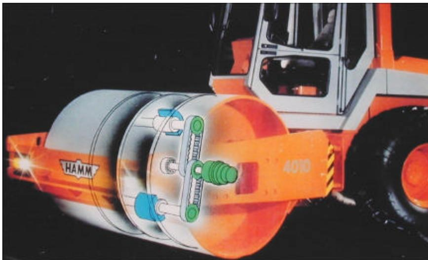
**Figure 5.** Oscillating roller.
