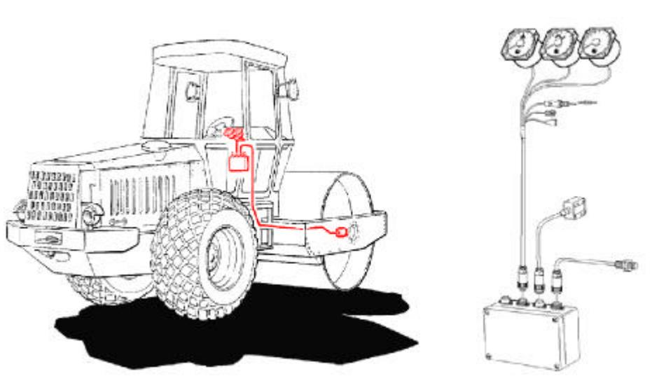
**Figure 4.** Compactometer components.
